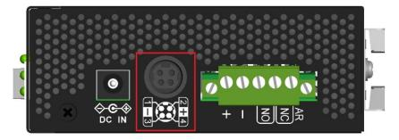
Connector: Female power DIN for external AC-DC power adapter
