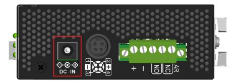
Connector: DC Jack (- $\emptyset$ 6.3mm/+ $\emptyset$ 2.0mm) for external AC-DC power adapter
