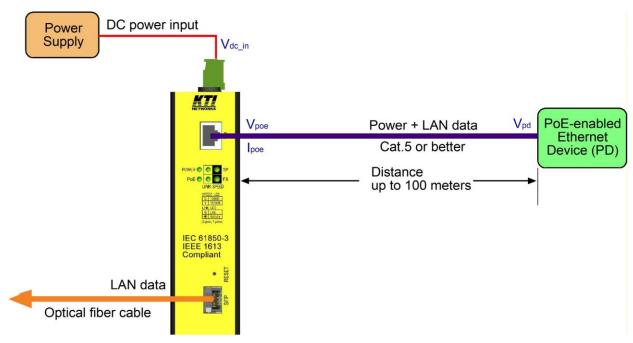
The device is equipped with PoE PSE function, which can supply power to a remote Ethernet device together with LAN data via TP port over Cat.5 cable. Above figure is a standard PoE connection example. By auto-detection and classification, the device supports the following PD types and classes:
