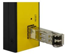
3. Until the SFP transceiver is seated securely in the slot, place the bail in lock position.
