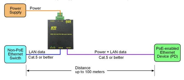
The cable distance including the segment from the injector to the Ethernet device and the segment to PD is no more than 100 meters.
