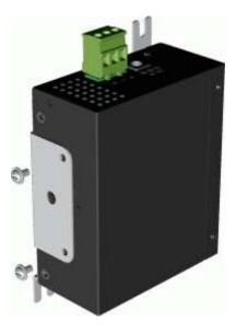
3. Screw the switch unit on a panel and the locations for screws are shown below:
