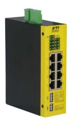
The switch provides eight 10/100/1000Mbps copper ports for connections to Ethernet, Fast Ethernet or Gigabit Ethernet devices. With the featured auto-negotiation function, the switch can detect and configure the connection speed and duplex automatically. The switch also provides auto MDI/MDI-X function, which can detect the connected cable and switch the transmission wire pair and receiving pair automatically. This auto-crossover function can simplify the type of network cables used.
