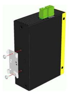
2. Attach bracket to the lower edge of the DIN rail and push the unit upward a little bit until the bracket can clamp on the upper edge of the DIN rail.
